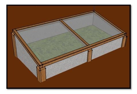
Cold frame concept using more advanced materials (insulated glazing and walls).
